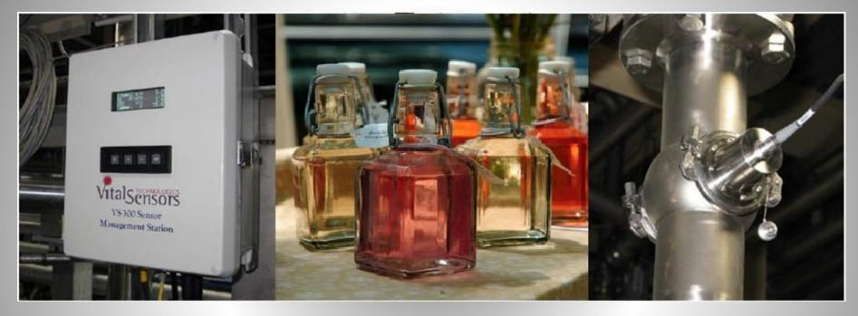
Real-time infrared instrument for process control
